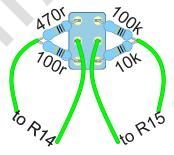
This is an additional mod you could add to the Green Screamer Deluxe, just take out two wires from the pads for R14 and R15 and wire it as its indicated on the graphic. This mod uses an extra toggle DPDT ON-ON.
