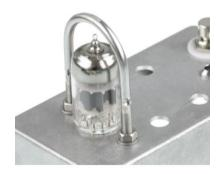
Don't forget to order a ceramic noval socket for your tube. The ones with the hole inside are perfect to fit your led and illuminate the tube.
