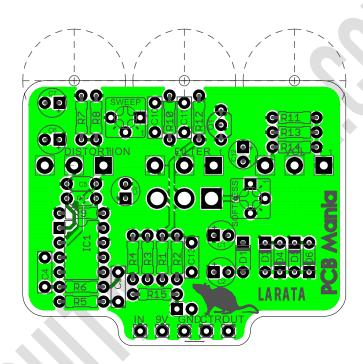
La Rata takes the maximum advantage of one of the most iconic drives, the Pro co's Rat. This board allows you to build many different verssions of this classic drive, from the 1978 original with the LM308 to the ones in current production. We also added the most popular mods on it, such as diode selector, Sweep control (the famous ruetz mode) and Softness control for the clipping section.
