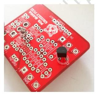
**Transistors\*\***: On the original unit it features a BC109C, this transistor silicon transistors on a can package for sure resembles to a germanium one, but its pure silicion. In my build I replaced it with a BC549, that's easier to find and considerably more affordable as well, here bellow you can see how to place it on board.
