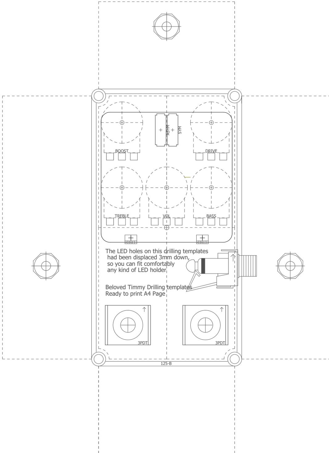
The LED holes on this drilling templates had been displaced 3mm down, so you can fit comfortably any kind of LED holder.
