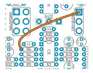
The second thing is to wire a cable from R6 to the Dry-blend Switch.
