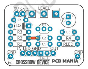
To keep it tidier, we recommend placing this resistor on the solder side and connecting it with c12 under the board.
