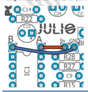
If using a MN3007 pad 'A' goes to GND and 'B' to 9v:
