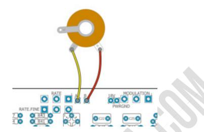
If you don't want to add the expression jack, you MUST place a jumper connecting the pads A and B to make the pedal work correctly.
