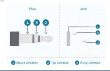
To add the expression jack, connect pad A with the TIP of the expression jack, pad B to RING, and leave SLEEVE unpopulated, as shown in the diagram below.
